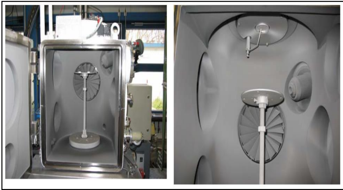
Fig.4- (a) Samples set-up inside the coating chamber,(b) the cathode position on the top of the coating chamber.
