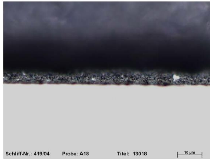
Fig.16- Coating morphology of sample "A", Optimal argon pressure:0.05 Pa average coating thickness: 6.28 μm.
